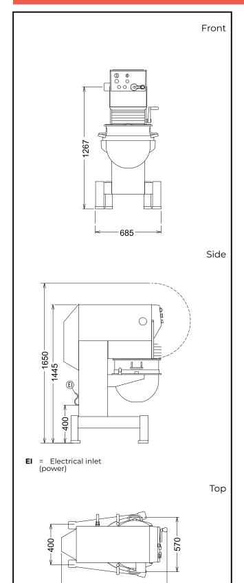
Electric 220-240/380-415 V/3 ph/50 Supply voltage: Electrical power, max: 1.54 kW **Total Watts:** 1.54 kW Capacity: ISO 9001; ISO 14001 kg/ Performance (up to): Cycle 60 litres Capacity: Key Information: External dimensions, 685 mm Width: External dimensions, 1087 mm Depth: External dimensions, Height: 1445 mm **Shipping weight:** 332 kg ISO 9001; ISO 14001 kg with Spiral hook **Cold water paste:** Egg whites: 100 with Whisk
